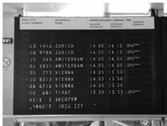
Figure 18. Broken flap display at the airport of Belgrade
