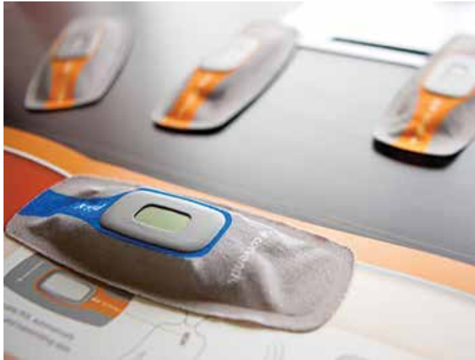
Figure 11. Smart bandages, including this one from Corventis, can transmit cardiac data in real time from a patient's body to their physician.
