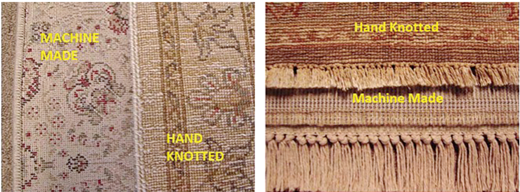
Figure 9. Differences between hand- and machine-made rugs
